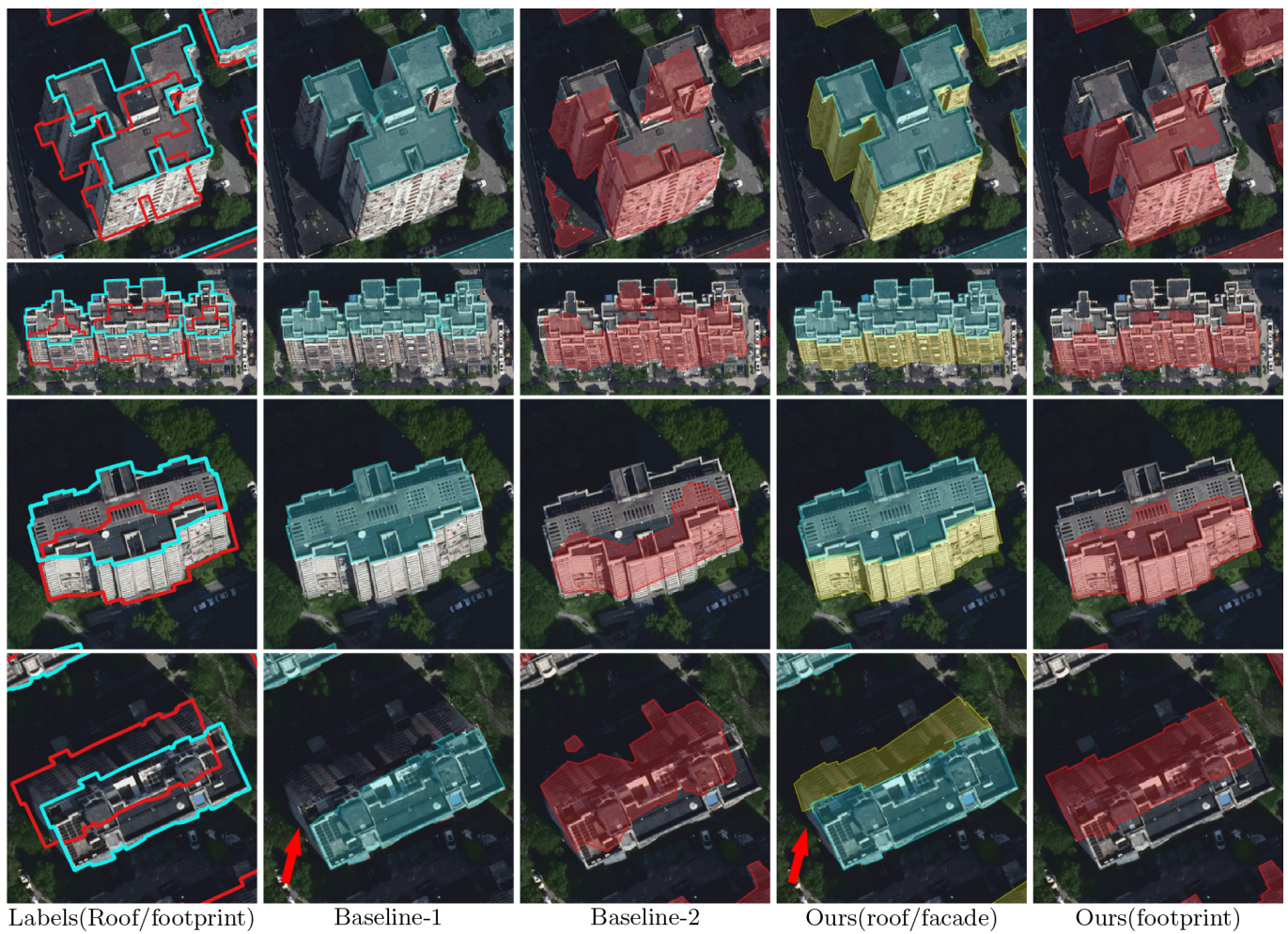
Figure 9. Results of the three workflows for typical high-rise buildings. The leftmost column shows the annotated roof and footprint labels of the test images, which are delineated by cyan and red polygons, respectively. The roof and footprint predictions of the three workflows are shaded in cyan and red on the images, respectively. The facade predictions of our workflow are also presented (in the fourth column, shaded in yellow).
