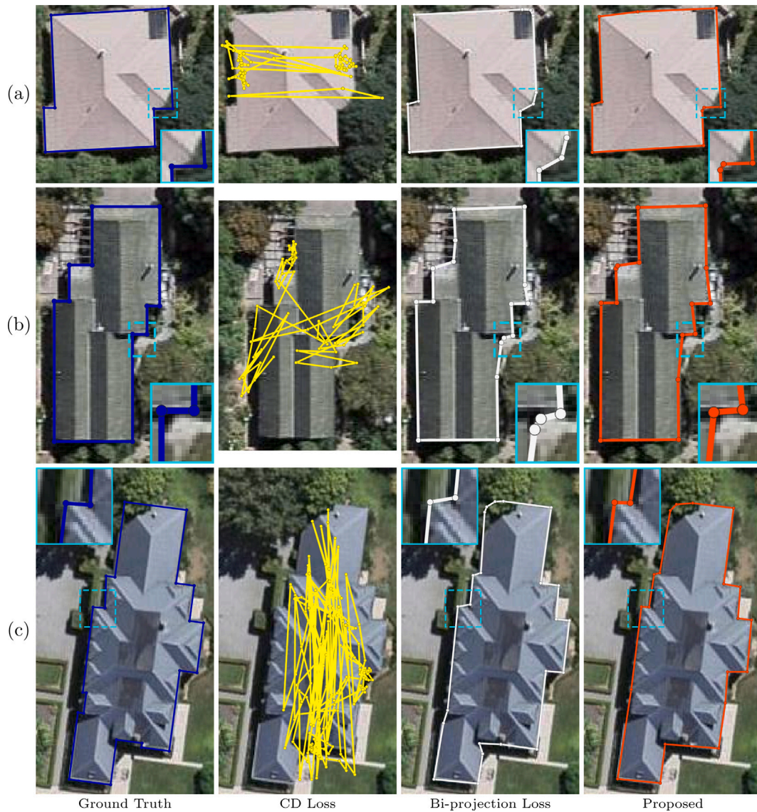
Fig. 8. Examples of the building vector results optimized by different loss functions. The ground truths, the vector results optimized by CD loss, bi-projection loss and the proposed scheme (bi-projection loss plus relative shape loss) are in blue, yellow, white and red, respectively. (For interpretation of the references to color in this figure legend, the reader is referred to the web version of this article.)
